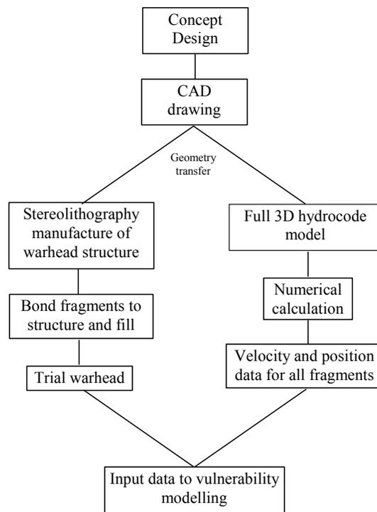
Figure 1 Integrated Concept Design Process
