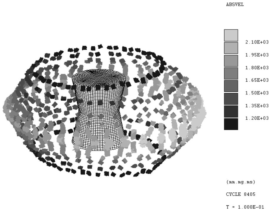
Figure 9 Absolute Fragment Velocity for Side Initiation Case at 100µs
