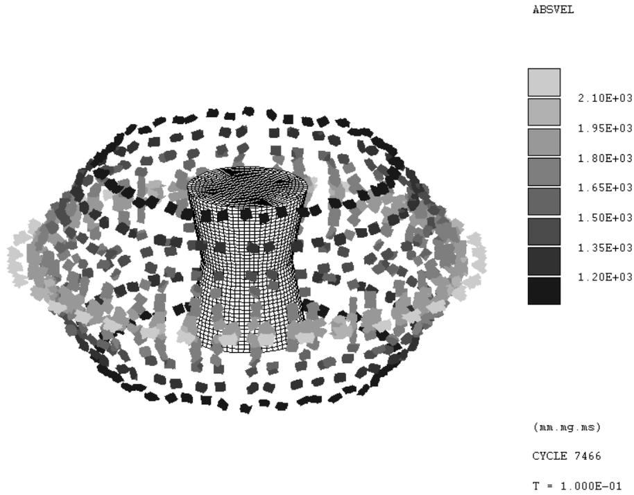
Figure 8 Absolute Fragment Velocity for End Initiation Case at 100µs
