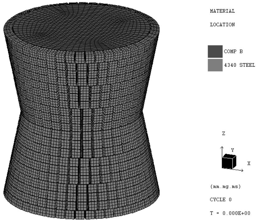
Figure 6 Example Warhead Geometry
