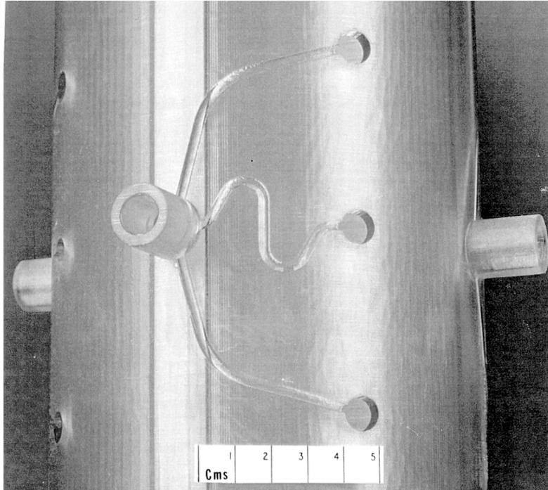
Figure 2 Rapid prototype component showing initiation tracks
