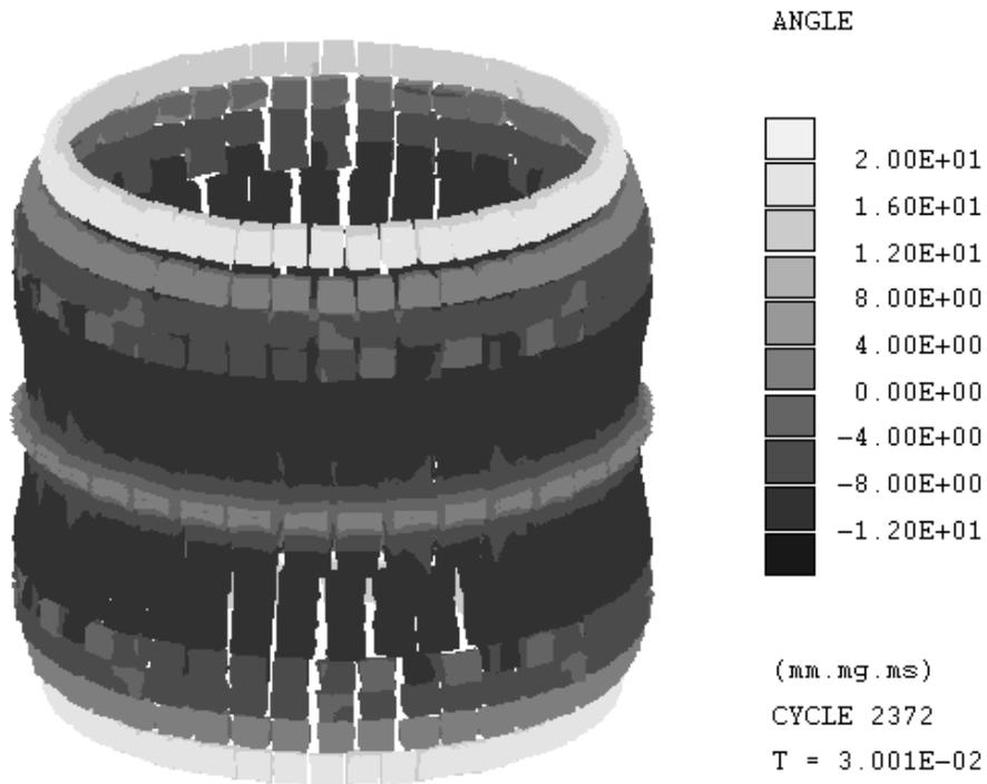
Figure 7 Fragment Ejection Angles for End Initiation Case at 30 $\mu$ s
