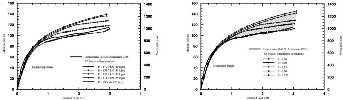
Figure 4. Connection response with varying pretension values(a); and varying friction coefficients (b).
