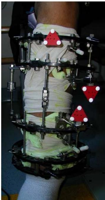
Fig. 2: To measure three-dimensional gap movement, triangles with three reflective markers each were mounted using custom-made clamps onto Schanz screws. The Schanz screws were detached from the fixator construct during the measurement sessions to allow direct measurement of fragment movements. The interfragmentary movements were determined from the rigid body movements of the triangles and the offsets toward the centre of the osteotomy gap.
