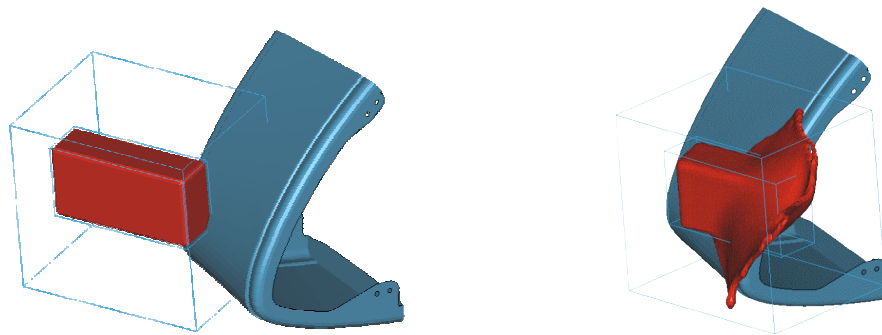
Figure 9. Simulation of a foam impact event using Eulerian Elements and an equation of state to represent the foam
