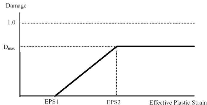
Figure 2. Cumulative Damage as a Function of Effective Plastic Strain
