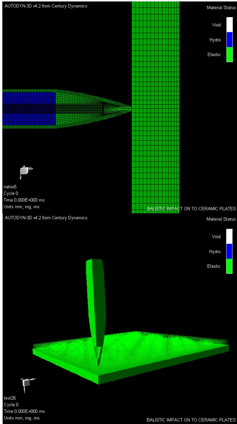
Figure 6. Full Lagrange and SPH models
