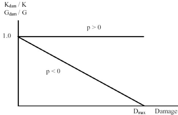
Figure 4. Bulk and Shear Modulus as Functions of Cumulative damage
