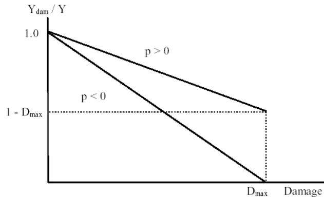
Figure 3. Yield Stress as Function of Cumulative Damage
