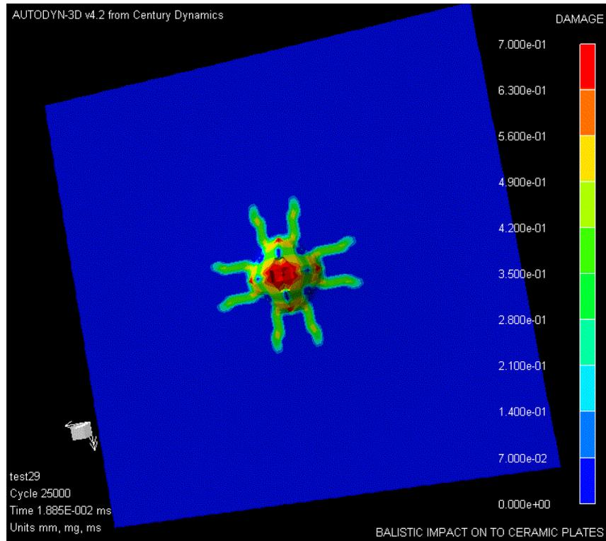
Figure 8. Crack propagation in Ceramic tile. Back view.
