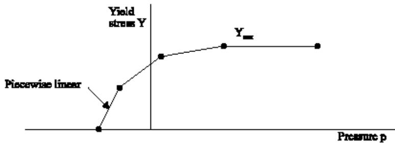
Fig 1. Mohr-Coulomb Model: Yield Stress as a Piecewise Linear Function of Pressure
