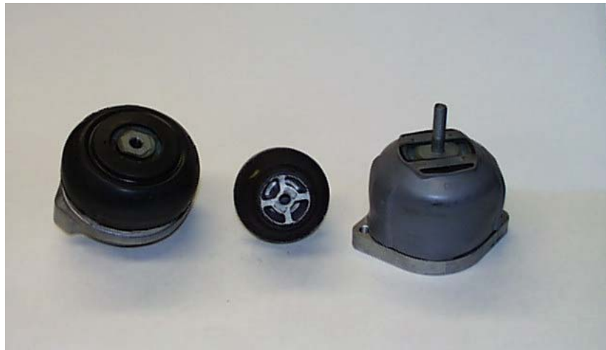
Figure 11. Rear Engine, Forward Engine and Transmission Mounts.
